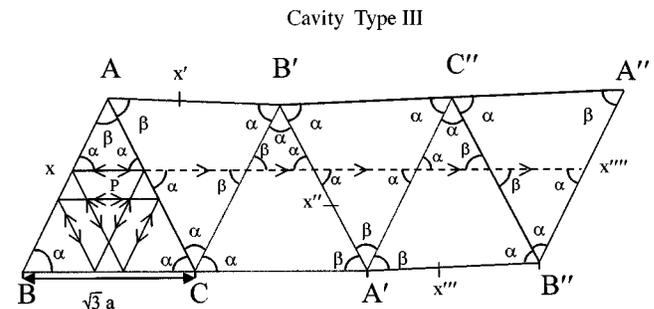
FIG. 4. WG-like cavity formed in a GaN pyramidal microcavity with a total optical path of about  $3\sqrt{3}an$ , where  $n$  is the refractive index of GaN.
