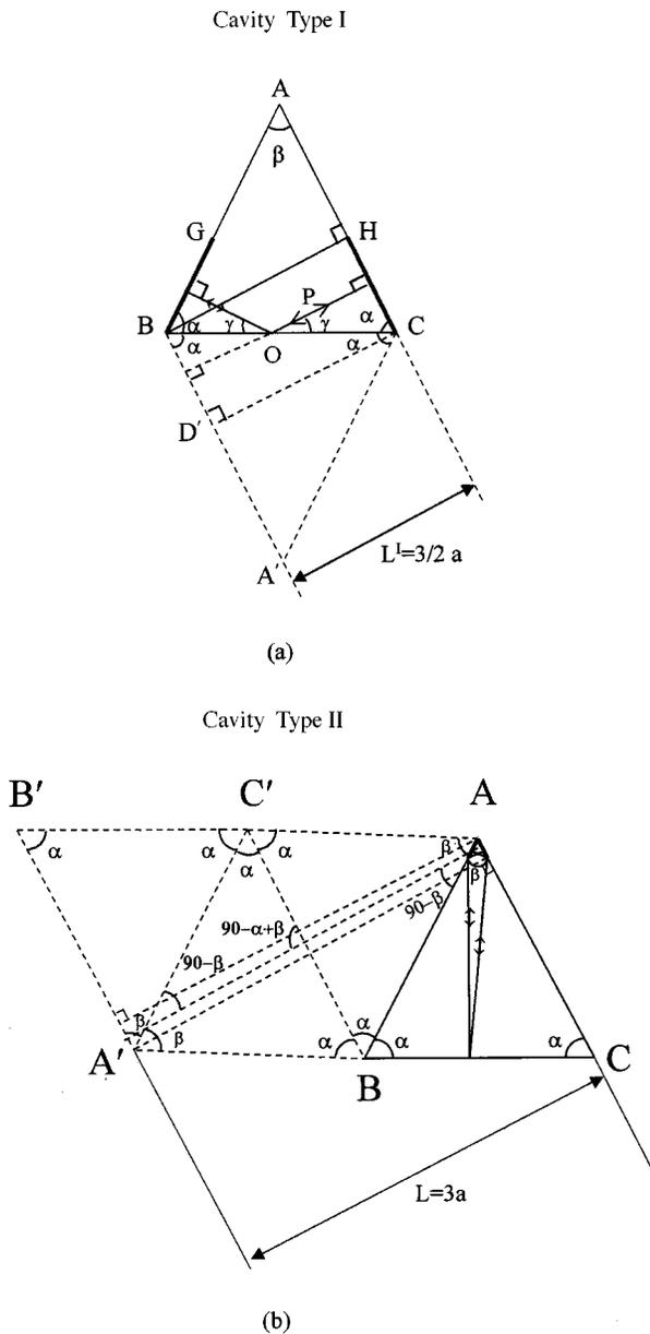
FIG. 3. Optical paths of Fabry-Perot-like cavities formed in a GaN hexagonal pyramidal microcavity determined by an optical ray tracing method. The effective optical path of (a) the first type optical resonance modes is about  $3an$  and (b) the second type optical resonance modes is about  $6an$ , where  $n$  is the refractive index of GaN.
