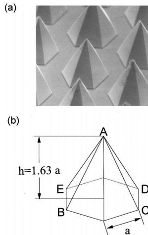
FIG. 1. (a) SEM image of an array of self-organized hexagonal GaN pyramids. (b) A schematic diagram of a single GaN pyramidal microcavity,  $a = 8.0\mu\text{m}$  and  $h = 1.63 a$ .
